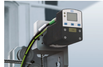
SIKO positioning drives ensure precise product position during the on-the-fly production change
