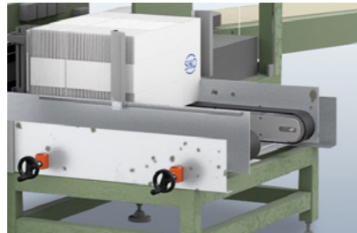
Reproducible adjustment of cardboard box erecting machines
