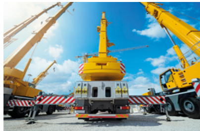
Position detection of the supports by draw-wire encoders and SGH sensors for the realization of a variable support base
