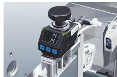
Height adjustment of label inspection
